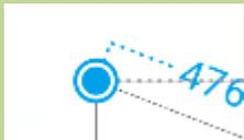
It indicates the position of current point. When specifying a point by tapping or dragging, as the finger lifting, the point marker appears.
